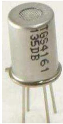
Figure 4. Carbon dioxide sensor.
